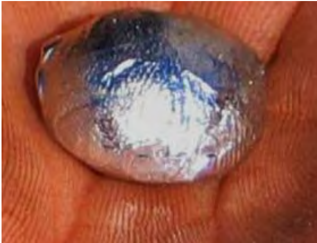
Figure 13. MERCURY-GOLD AMALGAM Soft bead of HgAu amalgam ready for firing off the mercury to leave gold. (photo: Peter Appel of GEUS)
