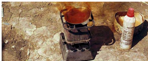
Figure 22. NITRIC ACID CLEANING Extremely toxic fumes being generated by hot concentrated nitric acid poured onto dry concentrate. After a few seconds the brown fumes are completely broken down to harmless nitrogen. Artisanal miners in Kyrgyzstan (photo: Peter Appel of GEUS)
