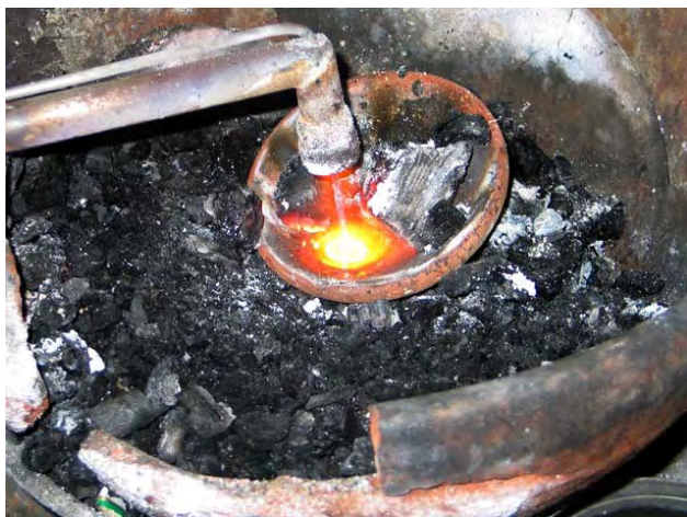
Figure 25. BORAX SMELTING Smelting concentrate to recover gold in the Philippines. (photo: Peter Appel of GEUS, Geological Survey of Denmark and Greenland)
