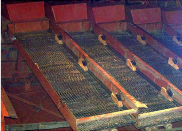
Figure 28. RUSSIAN EXPANDED METAL RIFFLES Sluice-boxes with expanded metal mesh riffles freshly installed in a Soviet bucket-line dredge in Mongolia. (photo: Robin Grayson)
