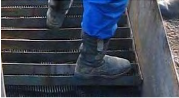
Figure 72. FLAT BAR RIFFLES Slanted flat bar riffles on ribbed rubber matting at a placer mine in the Zaamar Goldfield of Mongolia. (photo: Jeanie Barnett of GSA)
