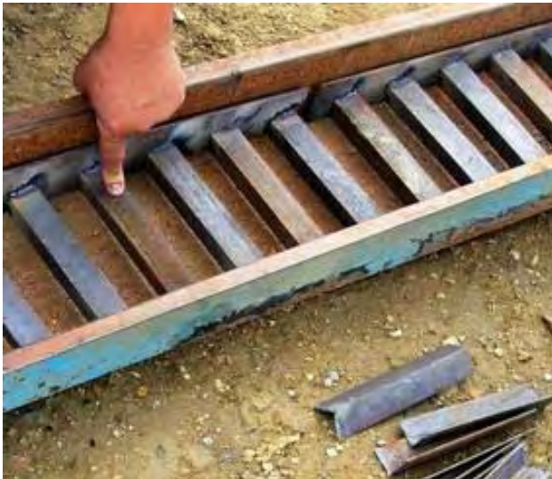
Figure 74. ANGLE-IRON RIFFLES A set of 1-inch riffled sluices being made 'on the spot' at the Sharin Gol mine of Polymet Potala Ltd in Mongolia. The welder has ensured each riffle has a 15° tilt. (photo: Robin Grayson)
