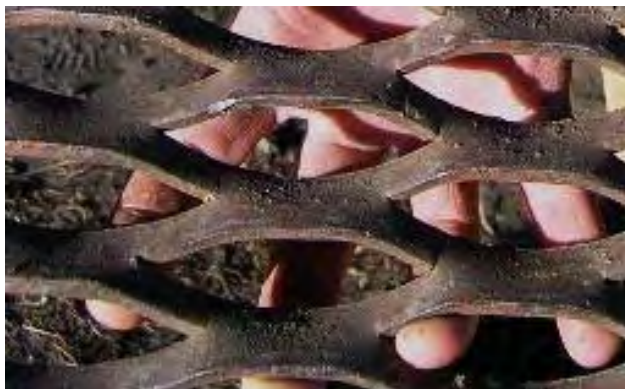
Figure 79. EXPANDED METAL GRATING RIFFLES Raised expanded metal grating suitable for using as large expanded metal riffles. (photo: Robin Grayson)
