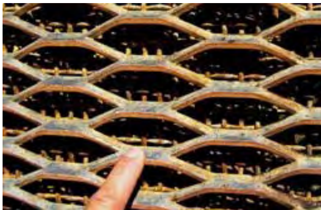
Figure 81. EXPANDED METAL MESH RIFFLES Raised expanded metal mesh suitable for using as small expanded metal riffles. (photo: Robin Grayson)
