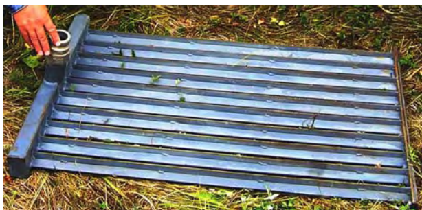
Figure 88. HYDRAULIC METAL RIFFLES A set of hydraulic metal riffles showing the manifold supplying the elutriation water under pressure. This set was manufactured by PAuSE Ltd in New Zealand. (photo: Robin Grayson)
