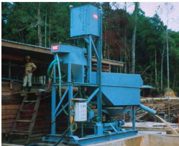
Figure 92. IHC JIG PLANT An IHC jig plant recovering fine gold in Sumatra, Indonesia. (photo: IHC Holland – www.ihcholland.com)
