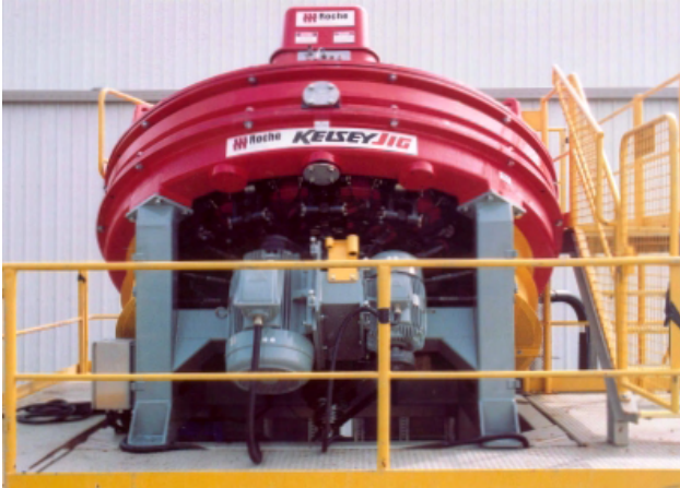
Figure 101. KELSEY CENTRIFUGAL JIG A model J1800 Kelsey centrifugal jig. (photo: courtesy of Dale Henderson of makers Roche Mining – www.rochemt.com.au )
