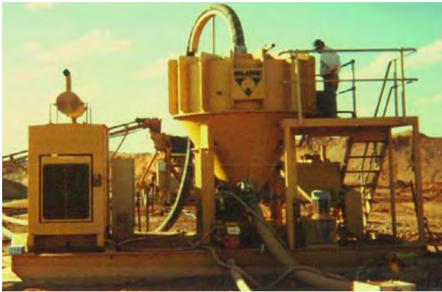
Figure 125. GEKKO™ IN-LINE PRESSURE JIG A skid-mounted IPJ at a placer gold mine in Australia. (photo: courtesy of Nigel Grigg of Gekko – www.gekkos.com)
