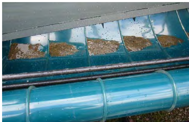
Figure 153. HPC HELIX BELT Material ascending the helix belt of the HPC-10 wash-plant. (photo: courtesy of Extrac-TEC www.extrac-tec.com )
