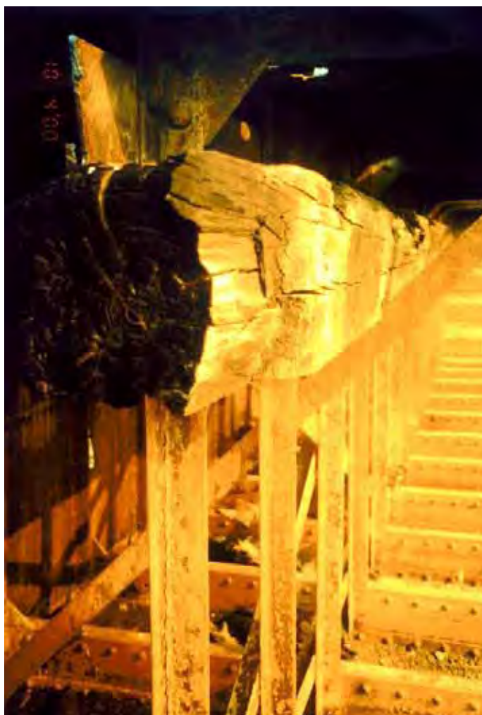
Fig.11: Timbers in sub-deck structure of English dredge. (Photographer: Iain Barclay, August 2000)
