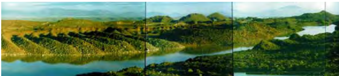
Fig.18: End result of the passage of the Monrosvestmet dredge at Zaamar, with creation of a series of arcuate mounds with large stones (oversize) on top of the fines. This artificial landscape was formerly the floodplain of the Tuul River. (photographer: John Farrington, August 2000).
