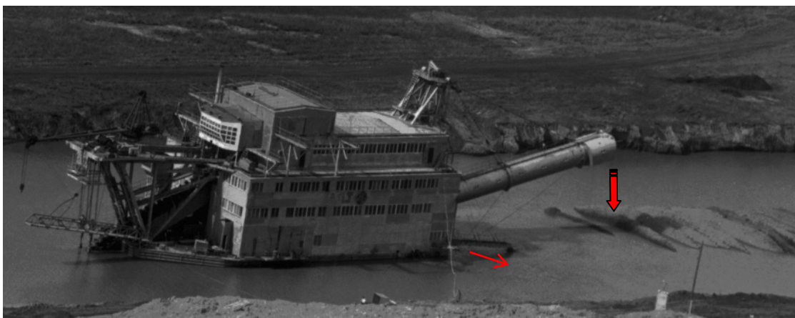
Fig.19: Closer view of Monrosvestmet dredge at Zaamar, mining from right to left. The fine-grained tailings are discharged by a pair of chutes, one of which is visible (thin red arrow), and the large tailings (oversize) are discharged by a conveyor on a boom (large red arrow). This causes the fines to be buried beneath a thick layer of large stones. (photographer: K.Dendinas, 1997).
