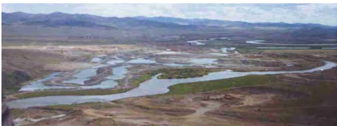
Fig.20: Major environmental disturbance caused by the combination of the Mongolrosvestmet gold dredge and associated drag-line. Dispensing with the drag-line and using a cutter-suction dredge would reduce the impact. Backfilling of the dredge ponds with the overburden mounds would be very expensive due to access by dragline now being blocked by dredge pools and unstable wet ground. The scope for creating a wetland mosaic with potential for significant wildlife gain is apparent.
