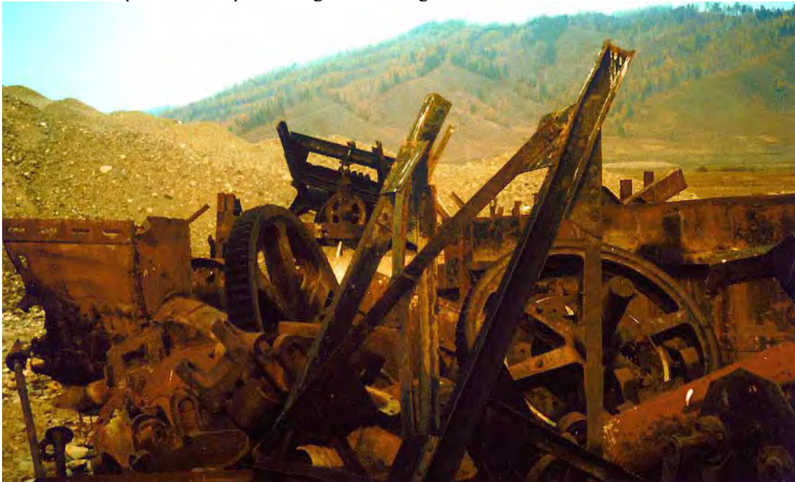
Fig.10: Winches and pulleys of the English dredge in Berleg Goldfield, awaiting assembly.
