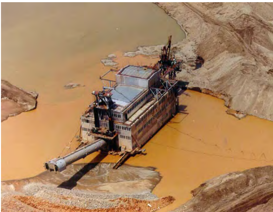
Fig.4: rear view of Mongolrosvestmet gold dredge showing disposal of coarse and fine tailings.
