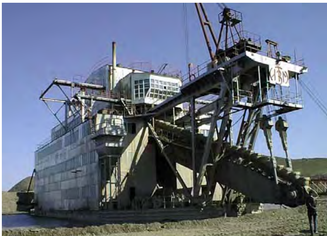
Fig.1: Mongolrosvestmet gold dredge in Zaamar Goldfield in 1998. The bucket-line is out of the water.
