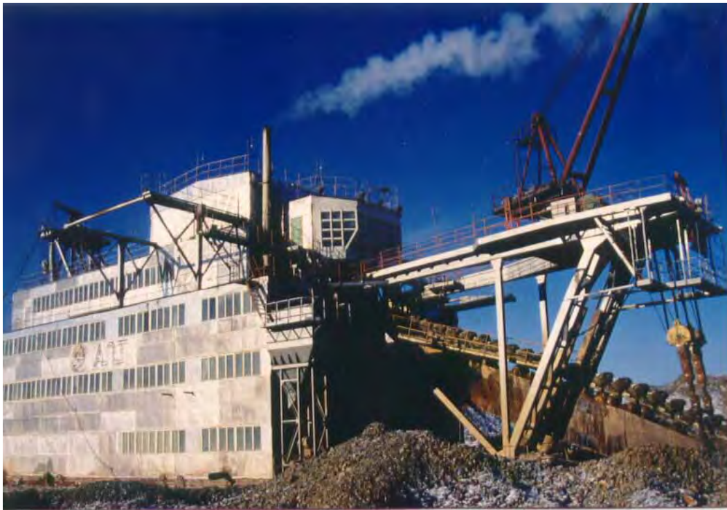
Fig.3: side view of Mongolrosvestmet gold dredge showing walled-in flanks to protect from cold.
