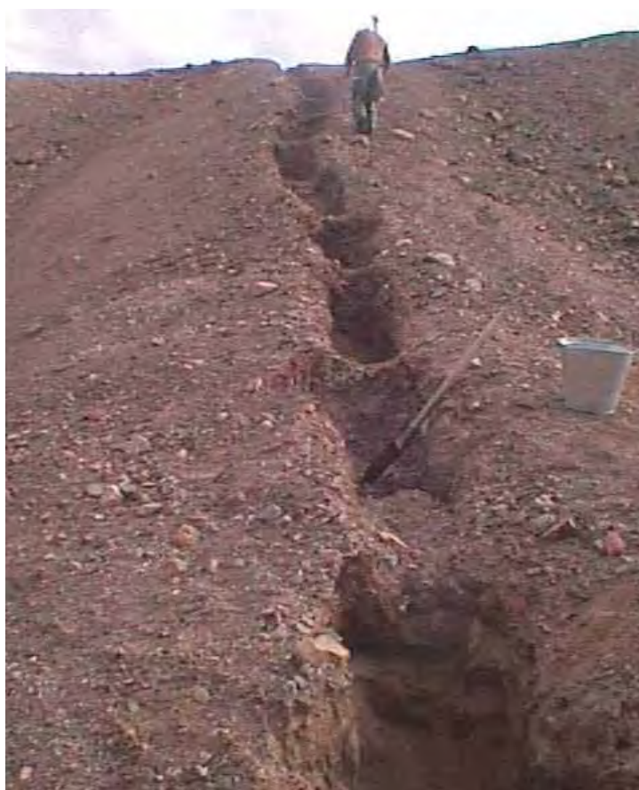
Fig. 2: Trenching by EMI through Upper Cretaceous gold/platinum conglomeratic placers near Altan Uul.
