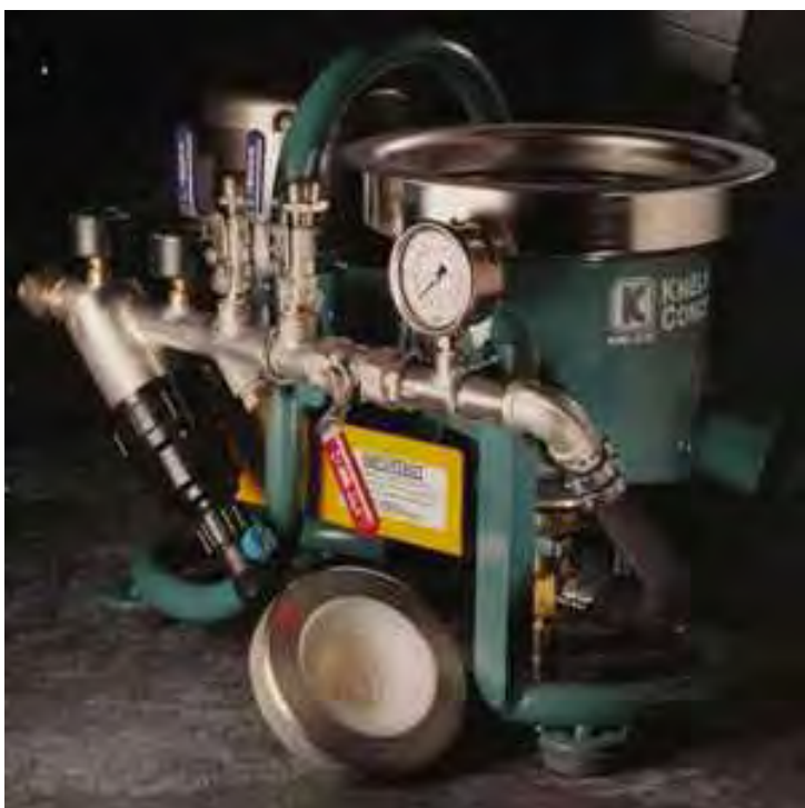
Fig.2: 3-inch KNELSON™ concentrator, with its centrifugal ribbed cone removed and placed in the foreground. (Photo: courtesy of Knelson Inc.)
