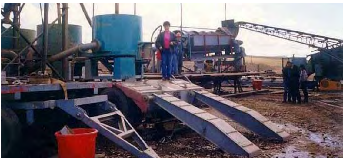
Fig.4: Closer view of KNELSONs™ at the Toson Terrace Mine, showing trommel.
