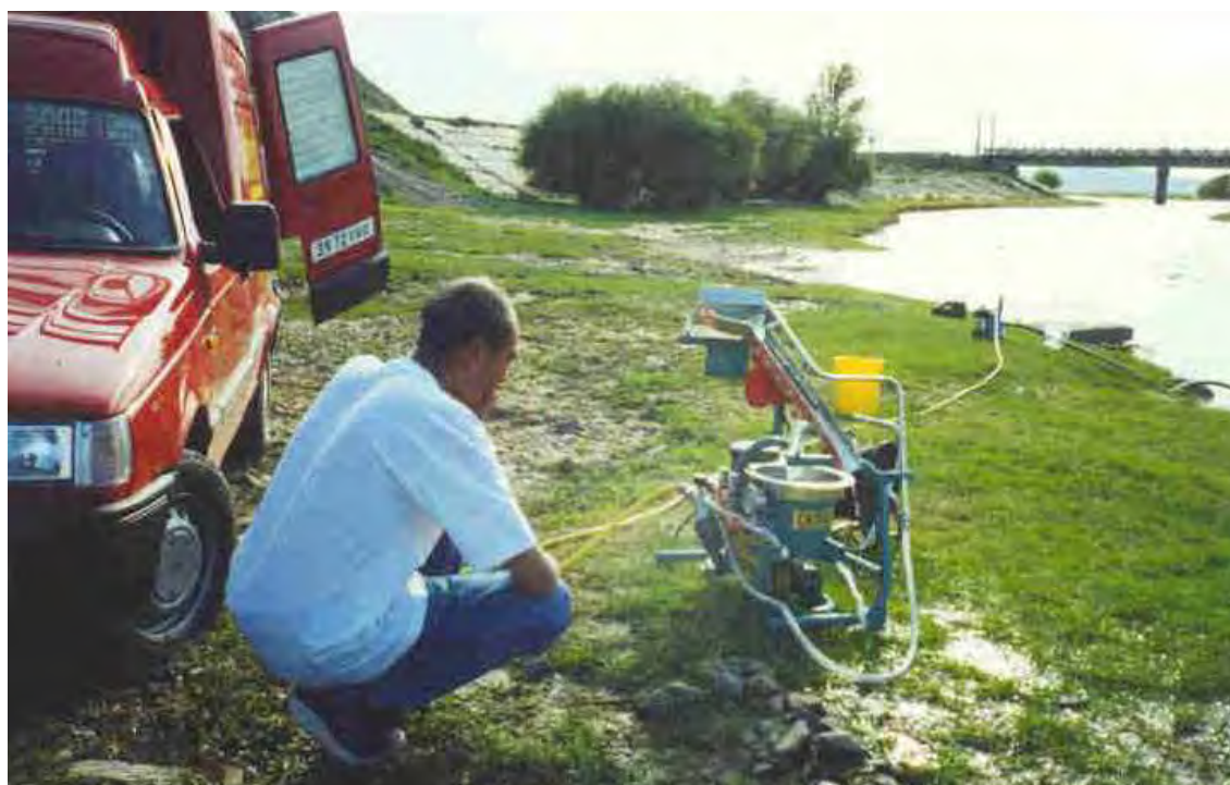
Fig.1: 3-inch KNELSON™ centrifugal concentrator undergoing testing at the Tuul River in 1998. Later it was used for laboratory testing of samples taken in winter from the Ikh Alt Mine.
