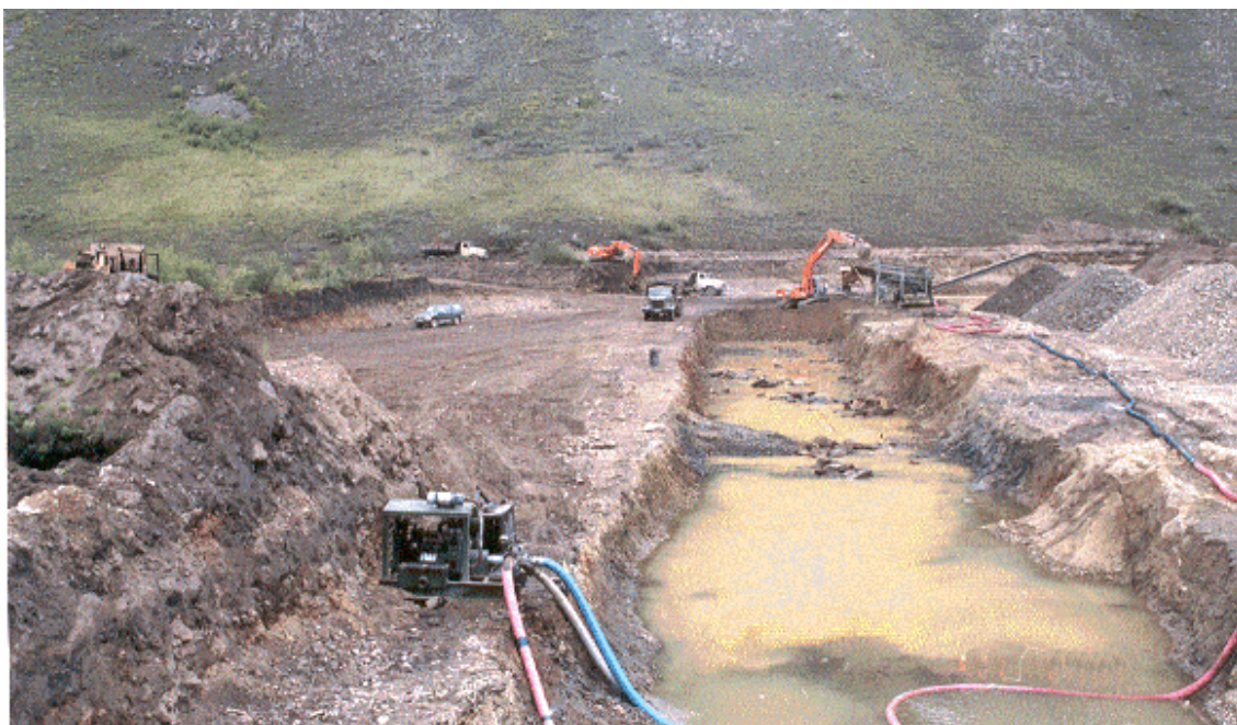
Fig.9: View of CGM's Yalbag Mine, showing a Hitachi excavator removing overburden (centre left) to expose the top of the placer, and a second Hitachi excavator (centre right) mining the placer and feeding it directly into CGM's 60m 3 /hour screen plant. Note the conical mounds of oversize dumped by conveyor. The string of oversize mounds results from the periodic moving of the skid-mounted mobile 60m 3 /hour screen plant to keep up with the advancing mining cut.
