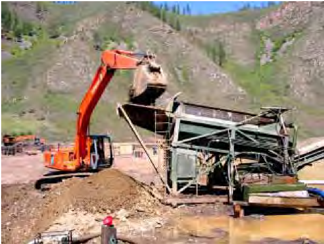
Fig.10: Mining operations at CGM's Yalbag Mine in the 2001 season. Direct mining of virgin placer is underway by a Hitachi excavator, swinging to load the pay gravel directly into the hopper of the skid-mounted New Zealand screening plant. No trucking is required.
