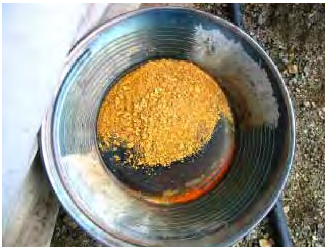
Fig.1: Gold concentrate in a gold pan, taken from the New Zealand hydro-active riffles in the 2001 mining season at CGM's Yalbag Mine in northern Mongolia.
