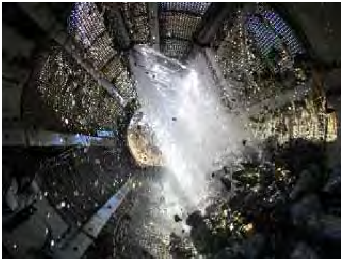
Fig.11: View inside the screen plant, rotating from left to right, showing the jetting of the tumbling pay gravel from 2 spray bars.
