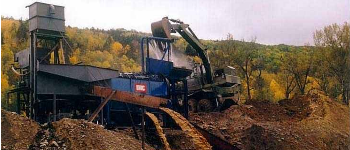
Fig.14: Ex-Soviet military 6-wheeled excavator (right) with 600-litre bucket dumping gravel into water-jetted Grizzly of IHC Conical Screen, feeding slurry to an IHC 2-Cell Jig (left) at the Bugant Mine. Note the clayey tailings issuing from the jig and water+oversize from the screen.
