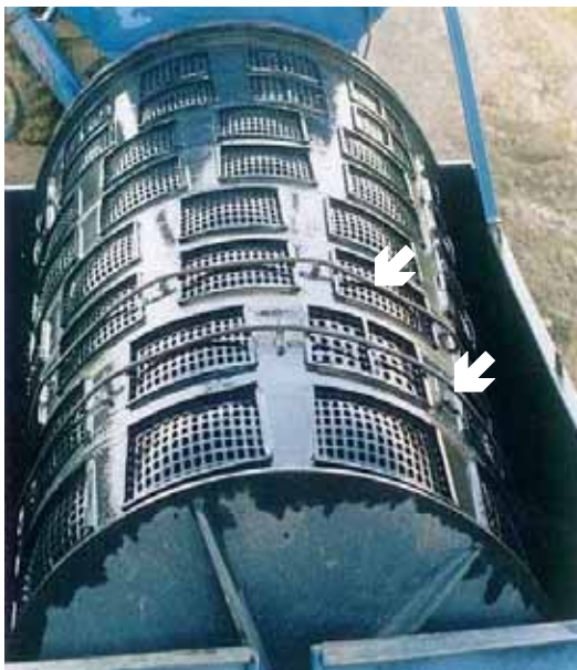
Fig.15: IHC Conical Screen showing outward buckling of the screen plates due to battering by slabs of oversize that got past the Grizzly. Arrows show the welded-on metal rods to prevent further buckling of screen plates.
