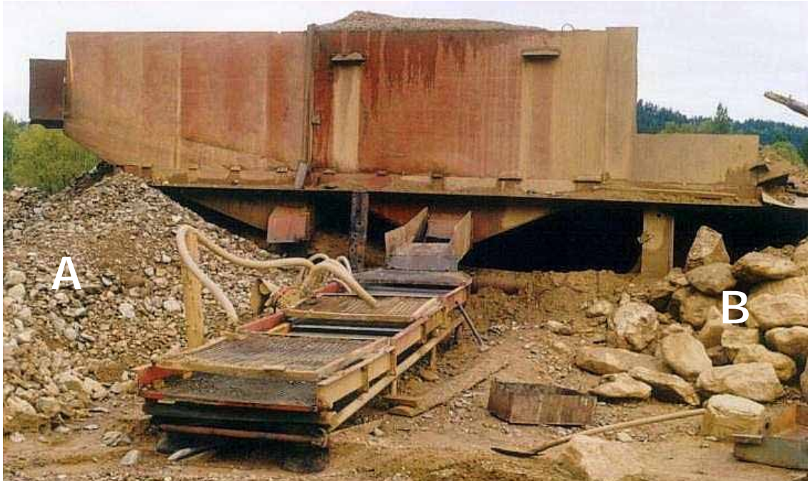
Fig.9: 25m 3 /hour PAuSE NZ Hydraulic Riffled Sluice fed via a link chute from a Russian-style static screen blasted by water cannon (right). A = a cone of oversize from the tail-gate of the screening box. B = large oversize manhandled away by the water cannon operator.
