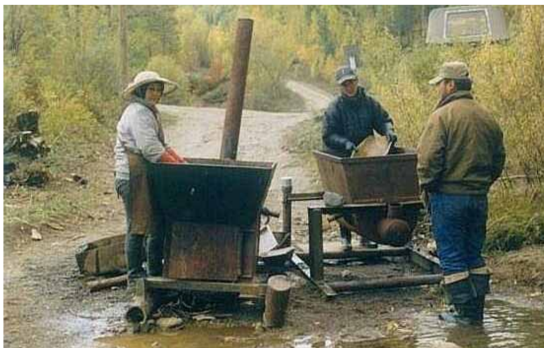
Fig.12: Upgrading concentrates by panning, led by the Chief Panner Mrs. Jadamba (left). A security guard looks on. The water is warmed by wood-fired boilers for comfort and accuracy.
