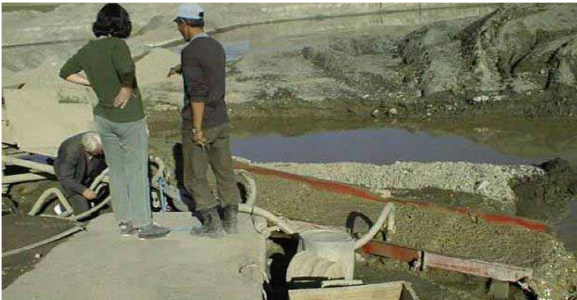
Fig.8: 25m 3 /hour PAuSE NZ Hydraulic Riffled Sluice in action in the Sergelen Goldfield at the Delger-Ech Mine. Note the 'steps' and bowing of the sluice due to lack of a supporting frame.
