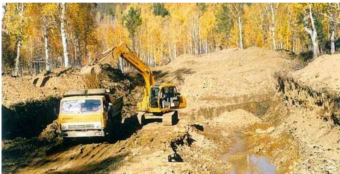
Fig.16: Korean Hyundai caterpillar-tracked excavator loading a Russian Kraz 5m 3 truck with placer at the Bugant Mine in 2001. The lack of clearance of trees and scrub was due to a decision to attempt high-grading at this location. The perpetuation of the Russian-style bulldozing of overburden into the forest destroyed 50% more trees than needs be, buried topsoil and sterilised some placer reserves. An influx of groundwater is invading the excavated area, counteracted by pumping.
