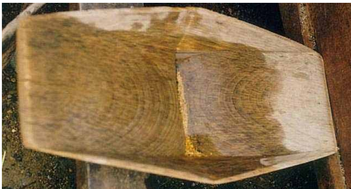
Fig.1: Gold recovered at Bugant Mine by the 25m 3 /hour PAuSE Hydraulic Riffled Sluice from New Zealand, revealed by upgrading in a traditional Siberian wooden gold pan.
