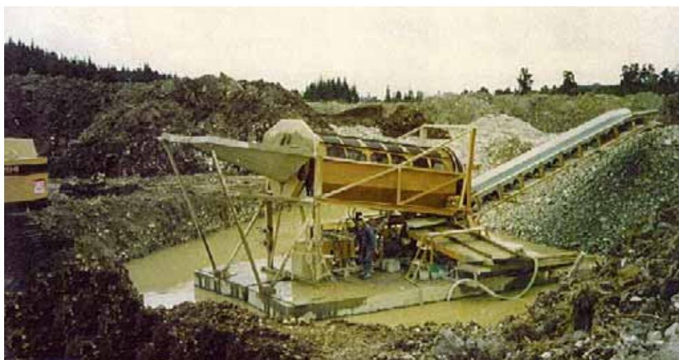
Fig.6: NZ Hydraulic Riffled Sluices, mounted on a pontoon in New Zealand. (photo: courtesy of Jim Loveridge)
