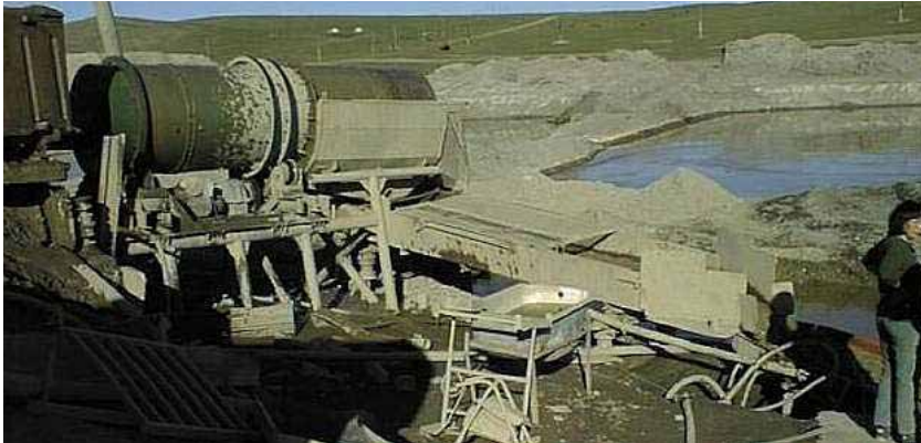
Fig. 7: Russian-style trommel and Russian-style sluice at the Delger-Ech Mine in the Sergelen Goldfield near Ulaanbaatar. Note the very large amount of sticky pervasive clay.
