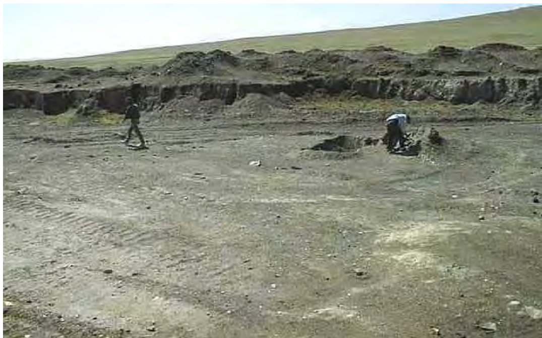
Fig.2: Elst Gold Mine in the Sergelen Goldfield. The mounds are of bulldozed thin overburden and topsoil, and the 'cliff' is the placer margin. The floor of the excavation is of shattered slatey bedrock. The small digging is of an illegal miner seeking gold in the shattered bedrock.
