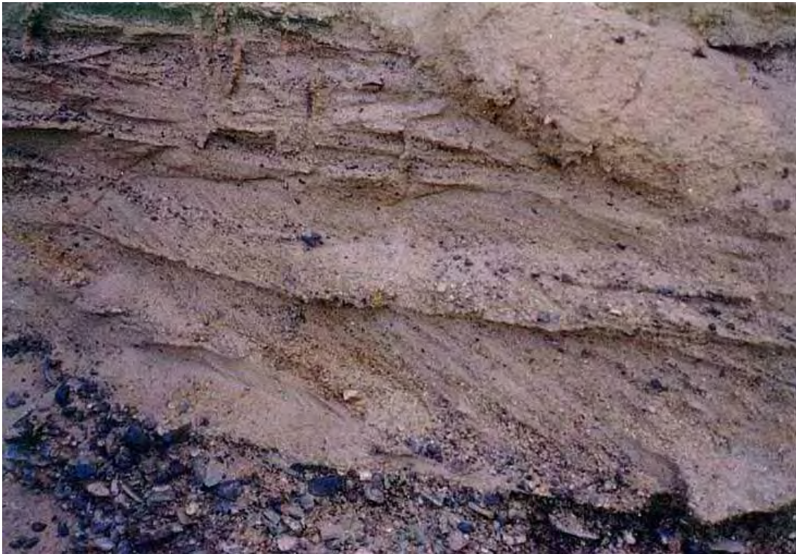
Fig.3: Cross-bedded well-rounded well-sorted fluvial placer exposed in the Toson Mine of Java Gold Corporation (JVAG on CDN), Toson Terrace, Zaamar Goldfield.
