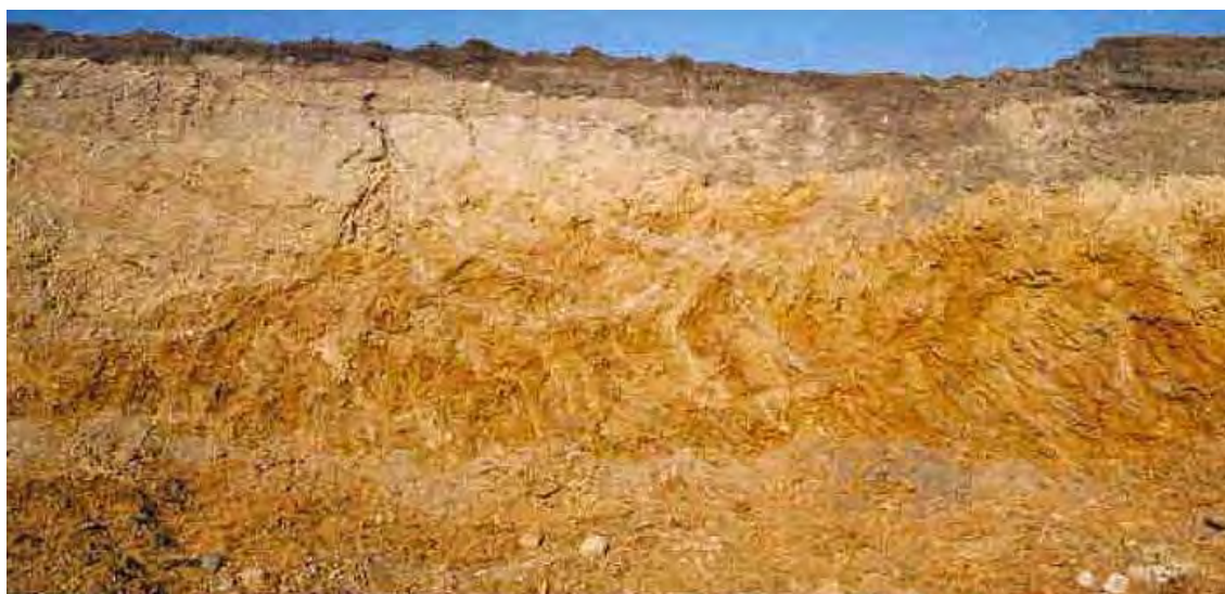
Fig.1: Solifluction placer exposed in the working face in of the Elst Mine in the Sergelen Goldfield. The view is up-valley, to the north-east. Note the partial overturning of relict bedding in the weathered broken bedrock, indicating substantial creep from the valley side on the left (north-west).
