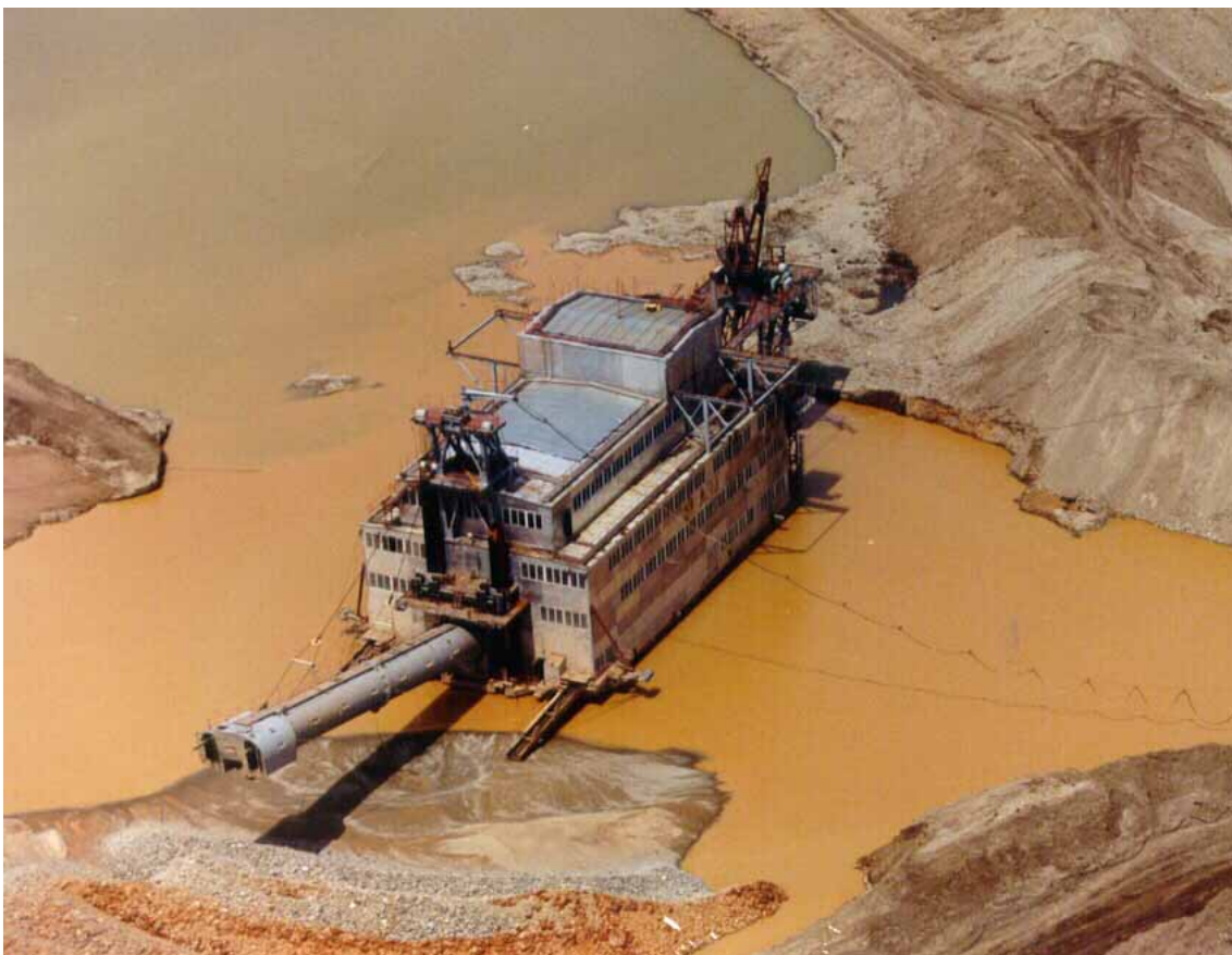
Fig.8: Rear view of the 'Alt' Gold Dredge showing disposal of coarse and fine tailings.
