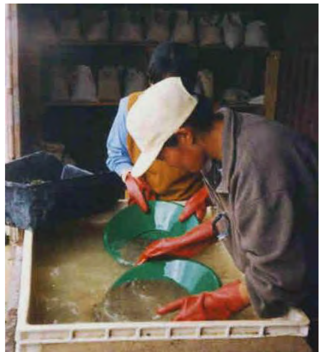
Figure 50. Comfortable posture using a North American gold pan requires a panning bath, in this instance an oblong water tank. Toson Terrace Mine of Java Gold Corporation in the Zaamar Goldfield of Mongolia. (photo: Robin Grayson)
