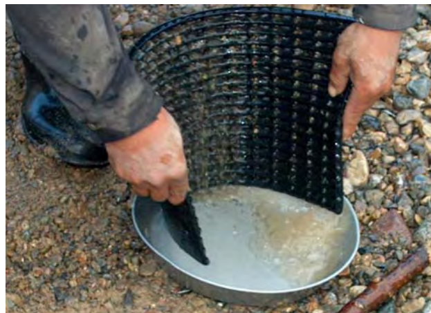
Figure 2. Artisanal miner loading concentrate from the ribbed rubber mat into an aluminium pan. Kyrgyzstan. (photo: Robin Grayson)
