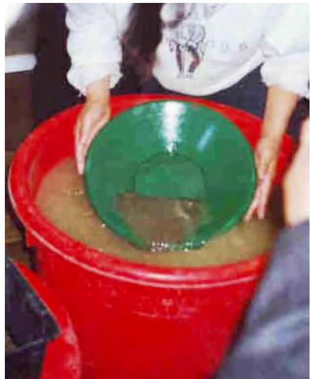
Figure 49. Comfortable posture using a North American gold pan requires a panning bath, ideally a round bath to snugly accommodate a round pan. Toson Terrace Mine of Java Gold Corporation in the Zaamar Goldfield of Mongolia. (photo: Robin Grayson)
