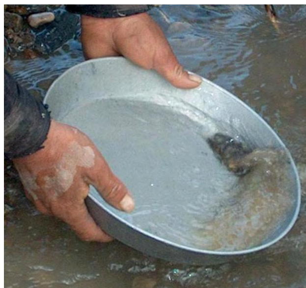
Figure 3. Panning in the same manner as for the North American Gold Pan. Kyrgyzstan. (photo: Robin Grayson)
