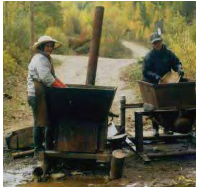
Figure 5. Provision of water baths allows lotok operators to maintain an upright posture. The water is kept warm by a wood-burning fire under the tank. Smoke is removed by the chimney pipe. Bugant Mine in north Mongolia. (photo: Gerrit Bazuin of Ochir LG Ltd)
