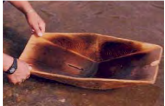
Figure 3. A lotok held steady with its v-depression horizontal and both the trays inclined towards it. This lotok has recently been cleaned by firing it. (photo: Robin Grayson)
