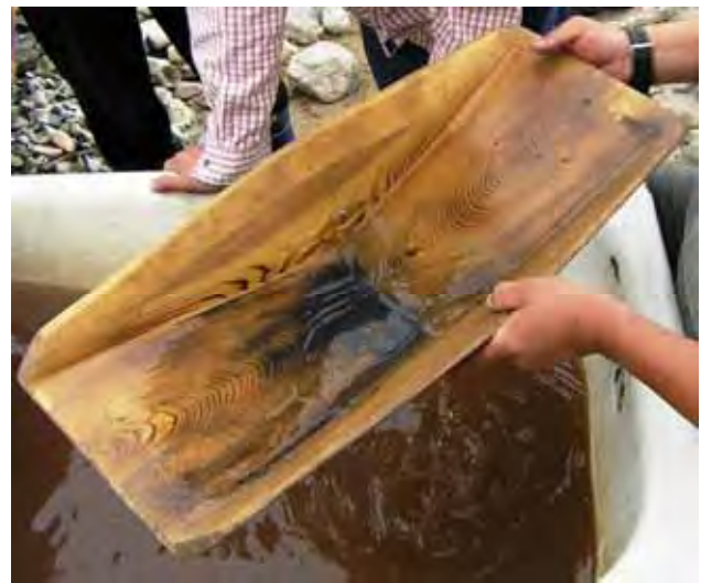
Figure 23. Minjin Batbayar holding a lotok clear of the water in the bath in order to inspect the contents. The process is slowed and then halted by the lifting action. (photo: Robin Grayson)
