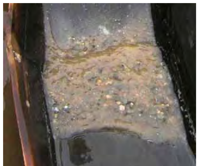
Figure 25. Nick Grayson has produced a pair of static waves caused by the underflow towards the v-depression when he tilted the lotok to a symmetrical horizontal position. (photo: Robin Grayson)
