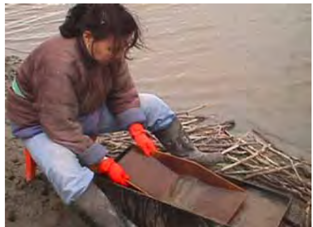
Figure 6. For prospecting, water baths are cut to the minimum size and the lotok according narrow. Warm water can be added from a kettle. The operator sits on a tiny stool. Altanzul of Eco-Minex is showing how to do it. (photo: Dr. Baatar Tumenbayar)
