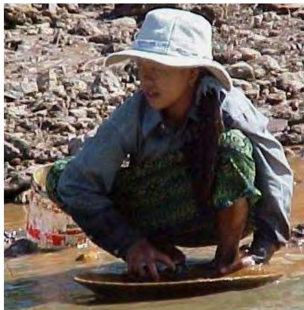
Figure 4. Even in an oblique side view the conical shape of the dulang is not apparent if the water is turbid. Mekong River in Laos. (photo: compliments of HoboTraveler.com – www.hobotraveler.com )
