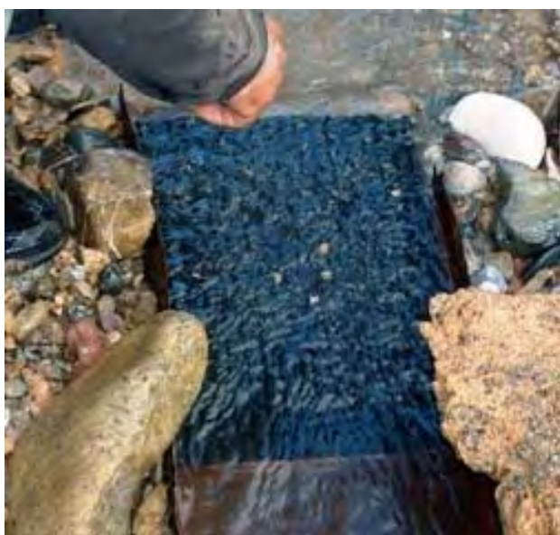
Figure 21. Re-inserting the ribbed rubber mat into the in-stream sluice. Note the prominent standing waves. (photo: Robin Grayson)
