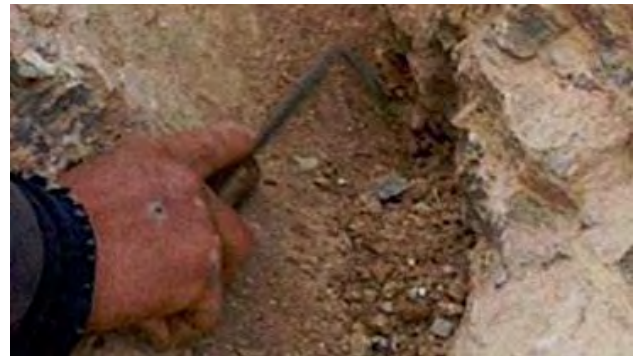
Figure 2. An artisanal miner using a modified metal bar ('oskar') to dislodge pay gravel from crevices of bedrock at the base of a mined-out placer. (photo: Robin Grayson)
