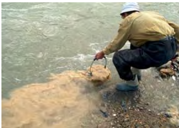
Figure 11. Bucketing underway, the miner lifting the bucket slightly to shed a plume of tailings in the midst of the tick-tock motion. (photo: Robin Grayson)
