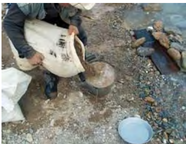
Figure 5. Artisanal miner pouring pay gravel from a sack into a bucket part-filled with water. The view showing all equipment – sack, bucket, gold pan, in-stream sluice and in the background a short stick for prodding the bucket contents. (photo: Robin Grayson)
