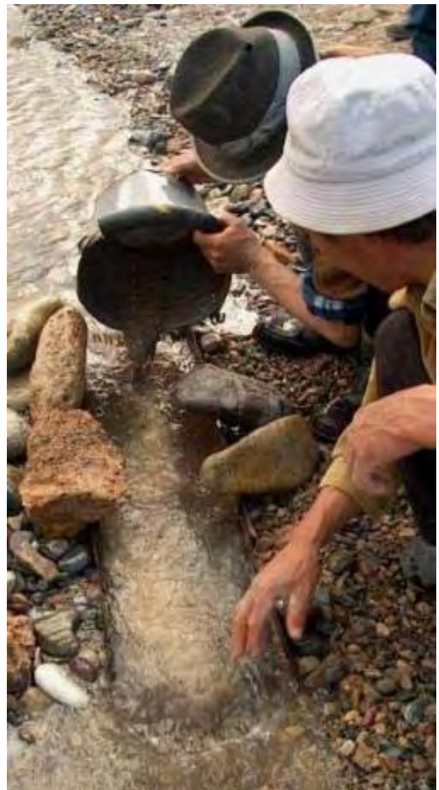
Figure 17. Slowly tipping the washed and winnowed contents of the bucket into an in-stream sluice down which a liberated plume of fines is racing. (photo: Robin Grayson)
