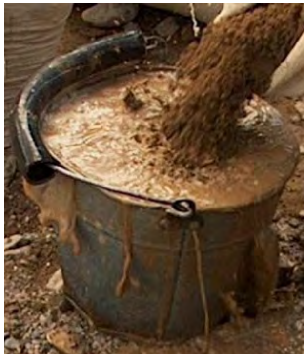
Figure 6. Although the pouring of dry pay gravel into the water ensures much turbulent wetting of the particles, it also risks ejecting valuable slurry over the sides, and in this instance through a rivet hole of the handle attachment. (photo: Robin Grayson)
