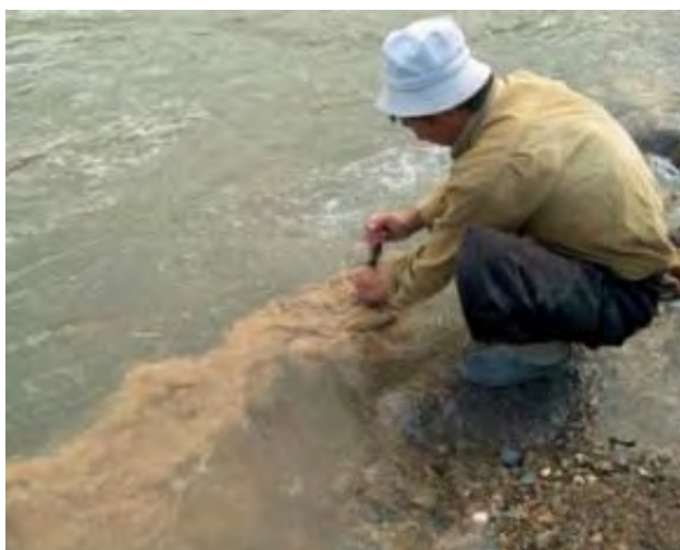
Figure 13. After a few minutes, the miner has ceased the tick-tock motion and lowered the bucket to rest on a submerged flattish boulder. He is now energetically mixing the contents of the pan using a stout short stick grasped in both hands. (photo: Robin Grayson)
