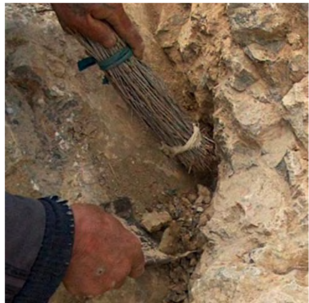
Figure 3. The same miner using a home-made brush to sweep the pay gravel into a plastic scoop for transferring into a cloth flour bag. (photo: Robin Grayson)
