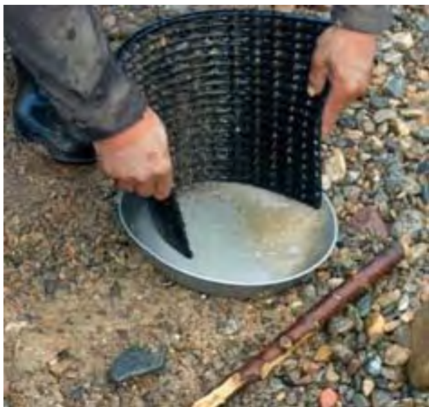
Figure 20. Loading concentrate from the ribbed rubber mat into a gold pan made from an aluminium fry-pan. (photo: Robin Grayson)
