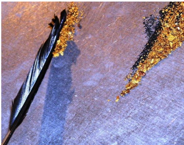
Figure 3. cleaning gold by blowing and with a feather Concentrate being cleaned by skilful use of a feather in the gold room of the Sharin Gol placer mine of Polymet Potala Ltd. Virtually all 135 placer mining companies in Mongolia use feathers, eliminating any need for mercury to clean the gold to a saleable concentrate. (photo: Robin Grayson)
