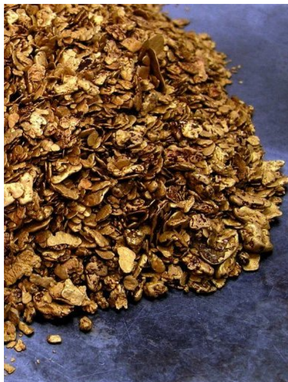
Figure 4. clean gold concentrate, after feathering Clean concentrate of Mongolian placer gold, ready for smelting to make a saleable dore gold ingot. Note the many flattish gold particles that are difficult to catch, yet each year over 10 tons of gold are recovered by gravitational means and finally cleaned by blowing and using a feather. Ar Naimgan Mine of Altan Dornod Mongol.
