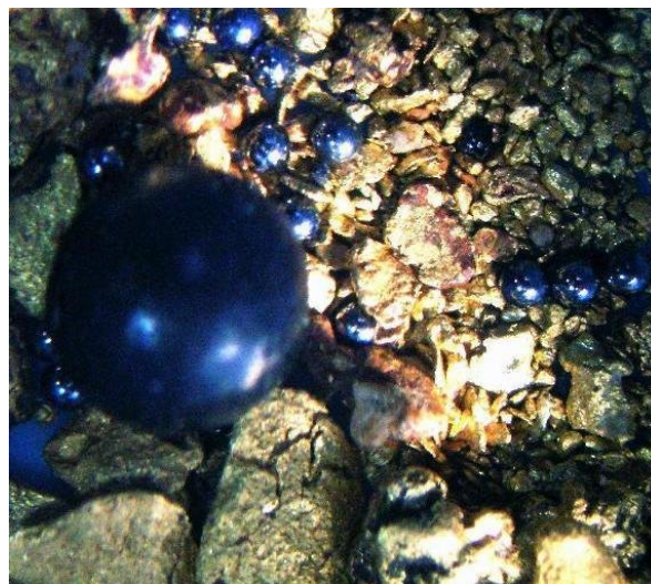
Figure 2. pen balls are smaller than lead shot Concentrate of placer gold, with over a dozen 0.5mm pen balls of tungsten carbide spheres dwarfed by a traditional tracer of 3mm diameter "bird shot" made of lead (Pb). (photo: Robin Grayson)
